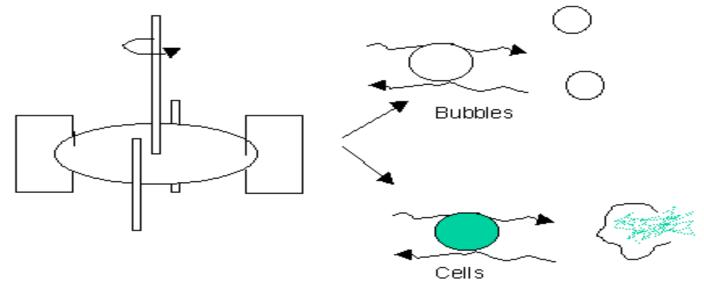
With radial flow impellers, vertical (or axial) mixing is achieved with the use of baffles
