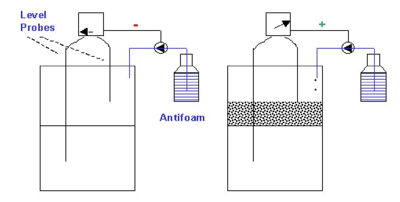
When the upper level probe is above the foam level, no current will pass between the level probes and the antifoam pump remains turned off. When the upper level probe is immersed in the foam layer, a current is carried in the foam. This causes the antifoam to turn on.
