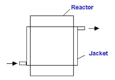
• The jacket will typically be "dimpled" to encourage turbulence in the jacket and thus increase the heat transfer efficiency.
