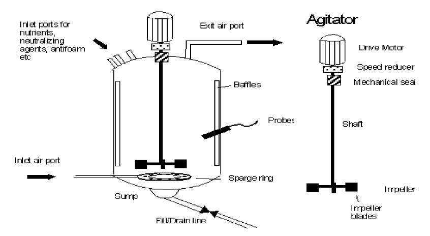
Laboratory scale bioreactors with liquid volumes of less than 10 litres are constructed out of Pyrex glass. For larger reactors, stainless steel is used.
