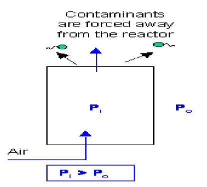
With aeration, positive pressure is always maintained and contaminants are pushed away from the reactor
