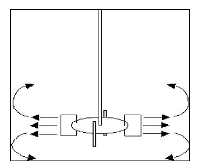
With radial flow impellers, the liquid is pushed towards the wall of the tank; that is, along the radius of the reactor
