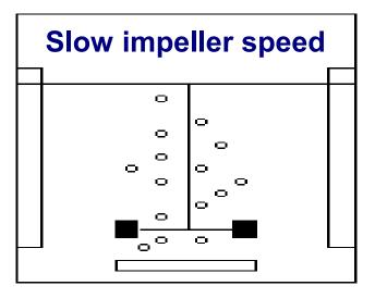
The bubbles will not be sheared into smaller bubbles and will tend to rise directly towards the surface
