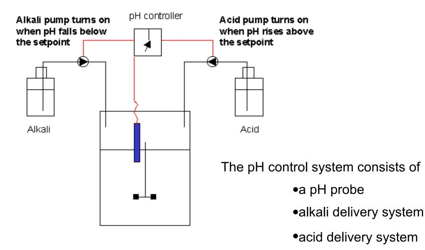
The pH probe is typically steam sterilizable
